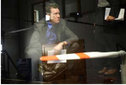
Patrick Graham of James W. Sewall Co. inspects a model turbine blade Thursday as it is subjected to winds of 4 mph in a wind tunnel at testing facility German WindGuard.
