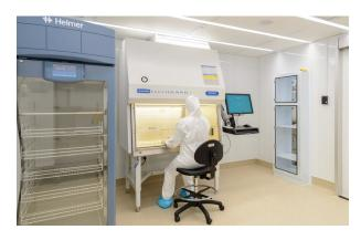
"In both of those settings, it's very important the work people are doing is kept free of contamination," says Eagleson. "Our product provides an enclosed space where the atmosphere is carefully controlled through products we engineer. There's a high efficiency filtration system in the cabinet and a fan system to move the air around in the way we've designed, offering protection for the product and the workers."
